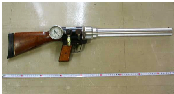
Fig. 2. Air gun used for attachment of the satellite tags from 2004 to 2008.
