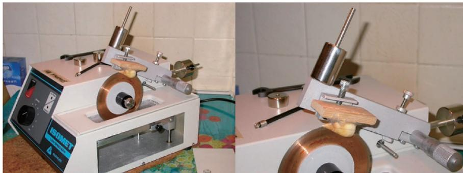
**Fig. 2.** Buehler Isomet low-speed diamond saw for sectioning teeth. The chuck and wood block mount for the tooth are shown. The tooth is affixed to the wood block using a standard hobby glue gun employing glue sticks. The glue is easily removed after cutting and can be made easier by soaking the tooth sections and block in water for some minutes.
