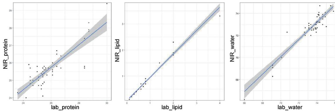
**Fig. 2.** Comparisons of biochemical components between laboratory-based and near-infrared (NIR) analyses to set a standard curve of the whale muscles for NIR spectroscopy. Left, protein; center, lipid; right, water. The muscle samples from Antarctic minke and North Pacific sei whales were used. The gray bands represent the 95% confidence intervals.
