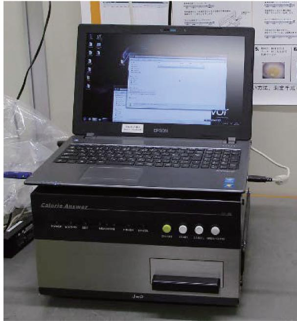
**Fig. 1.** Near-infrared spectrometer CA-HM (Joy World Pacific Co. Ltd.) and a terminal PC. The solid muscle samples were homogenized using a food processor and a portion the (approximately 25 g) was set for analysis on a saucer at the lower right slot.
