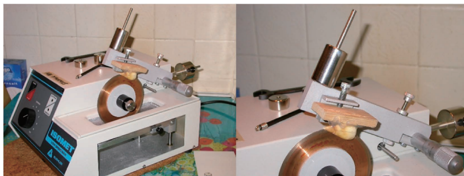
Fig. 2. Buehler Isomet low-speed diamond saw for sectioning teeth. The chuck and wood block mount for the tooth are shown. The tooth is affixed to the wood block using a standard hobby glue gun employing glue sticks. The glue is easily removed after cutting and can be made easier by soaking the tooth sections and block in water for some minutes.
