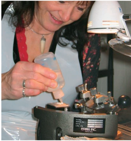
Fig. 3. A portable benchtop freezing microtome used for sectioning decalcified teeth. Note the horizontal cutting plane, the fixed freezing stage and the mobile blade. The specimen is frozen by means of a Peltier device with flowing water in counter current. The blade is not cooled and the microtome is operated at room temperature. The temperature of the freezing stage is generally around -12^{\circ}\text{C} and can be adjusted by altering the water flow to the device.
